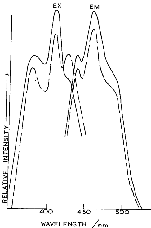
Fig. 1. Fluorescence excitation (EX) and emission (EM) spectra of 9,10-dihydroxyanthracene in n -hexane (deoxygenated) (—) and polypropylene film after thermal treatment with anthraquinone at 190°C for 1 min (- - -).
